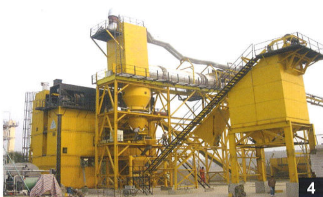
4 An asphalt batching plant with recycling facilities
