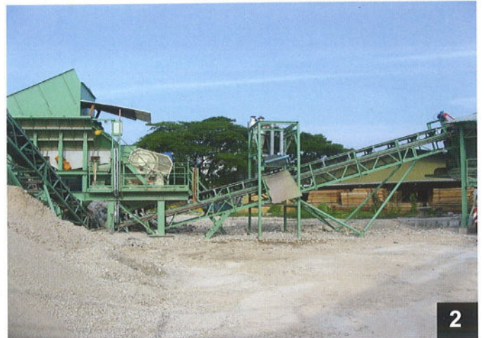
Preliminary crushing and removal of ferrous metals
