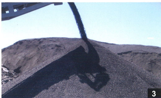
3 RAP is ready to be used
