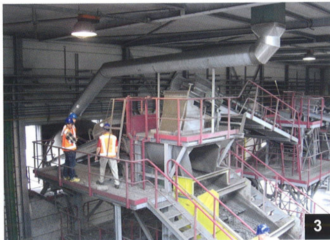
Crushing and screening of IBA
