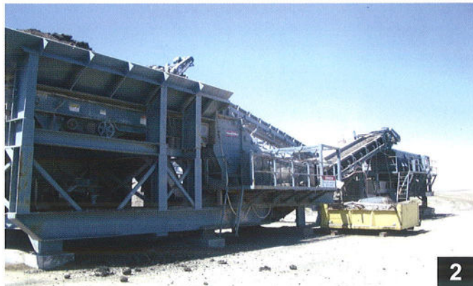
2 Crushing and screening of asphalt pavement waste
