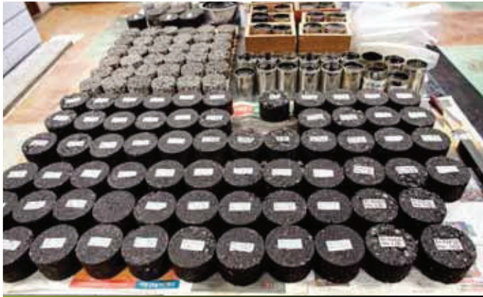
Waste materials (asphalt waste and incinerator bottom ash) transformed for use in road construction.
