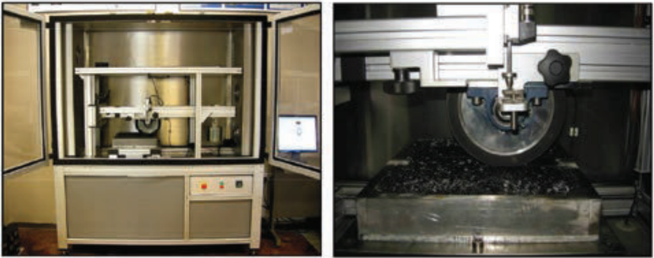
Figure 2: Wheel tracking machine (left) and close-up view of test sample (right)
