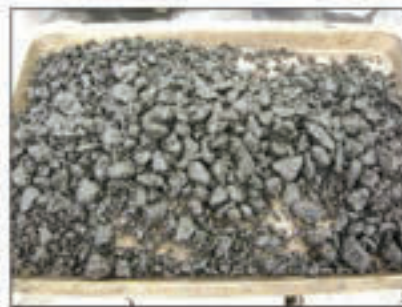
Figure 5: Uncompacted sample for G_{mm} measurement (left) and sample placed in a pycnometer (right)
