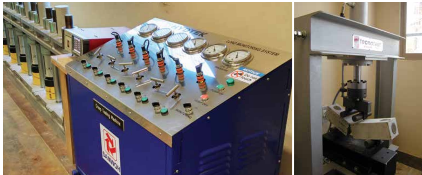
above, from left: Creep testing equipment developed by Samwoh Flexural strength testing
